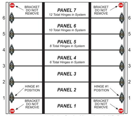
Inside view of overhead door with standard 2" rollers.
